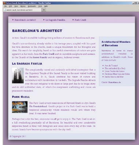
A A common layout with main navigation along the top, main content on the left, a sidebar on the right, and the footer at the bottom. CSS is required to make the page look like this.
